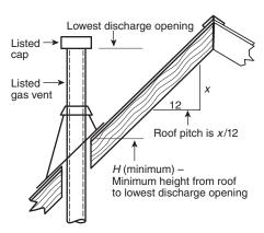
FIGURE 12.7.3 Termination Locations for Gas Vents with Listed Caps 12 in. (300 mm) or Less in Size at Least 8 ft (2.4 m) from a Vertical Wall.
