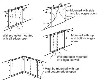
Wall protector installed in corner
