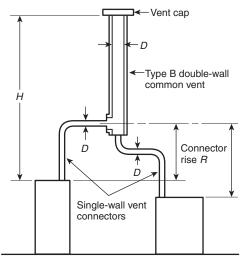
Table 13.2(b) is used when sizing single-wall vent connectors attached to a Type B double-wall
