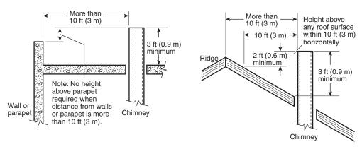
(b) Termination More Than 10 ft (3 m) from Ridge, Wall, or Parapet
