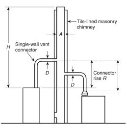
Table 13.2(d) is used when sizing single-wall metal vent connectors attached to a tile-lined masonry chimney.
