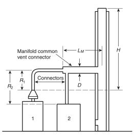
Example: Manifolded common vent connector  $L_M$  can be no greater than 18 times the common vent connector manifold inside diameter; that is, a 4 in. (100 mm) inside diameter common vent connector manifold should not exceed 72 in. (1800 mm) in length. (See 13.2.4.)
