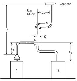
Asbestos cement Type B or single-wall metal pipe vent serving two or more draft hood–equipped appliances. [See Table 13.2(e).]
