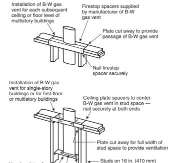
FIGURE 10.26.1.3 Installation of Type B-W Gas Vents for Vented Wall Furnaces.
