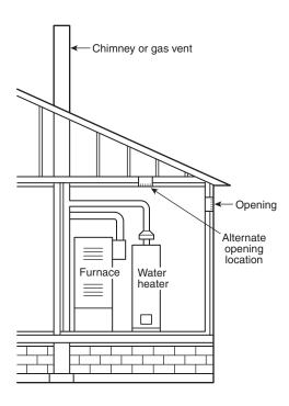
FIGURE A.9.3.3.2 All Combustion Air from Outdoors Through Single Combustion Air Opening.
