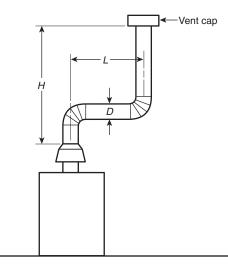
Asbestos cement Type B or single-wall metal vent serving a single draft hood-equipped appliance. [See Table 13.1(e).]
