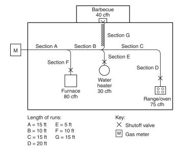
FIGURE B.7.4 Piping Plan Showing Modification to an Existing Piping System.
