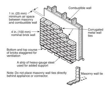
FIGURE 10.3.2.3(c) Masonry Clearance Reduction System.
