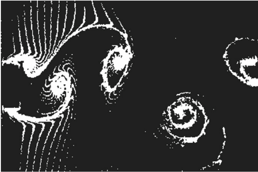
Fig. 6.4 Flow around rectangular cylinder, Reynolds number Re = 200 . From [114]
