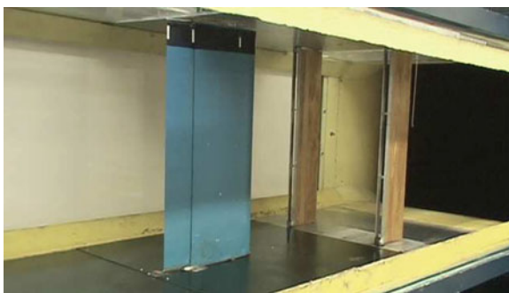
Fig. 14.6 Photograph of the experimental model with gust generator in the wind tunnel test
